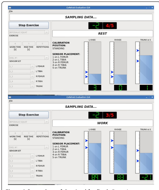
Figure 2 Screenshots of the visual feedback. Exemplary screenshots of the special interface used as visual feedback during the rest (top) and work (bottom) phases of the squat exercise. Users can monitor in real-time the knee (L KNEE and R KNEE) and thorax (TRUNK vs S, lunge and squat exercises only) flexion angles via bar plots and numerical values, and the desired target range by the position of the blue arrows. They can also have access (top of the screen) to the countdown (in green) and the repetition (red).
